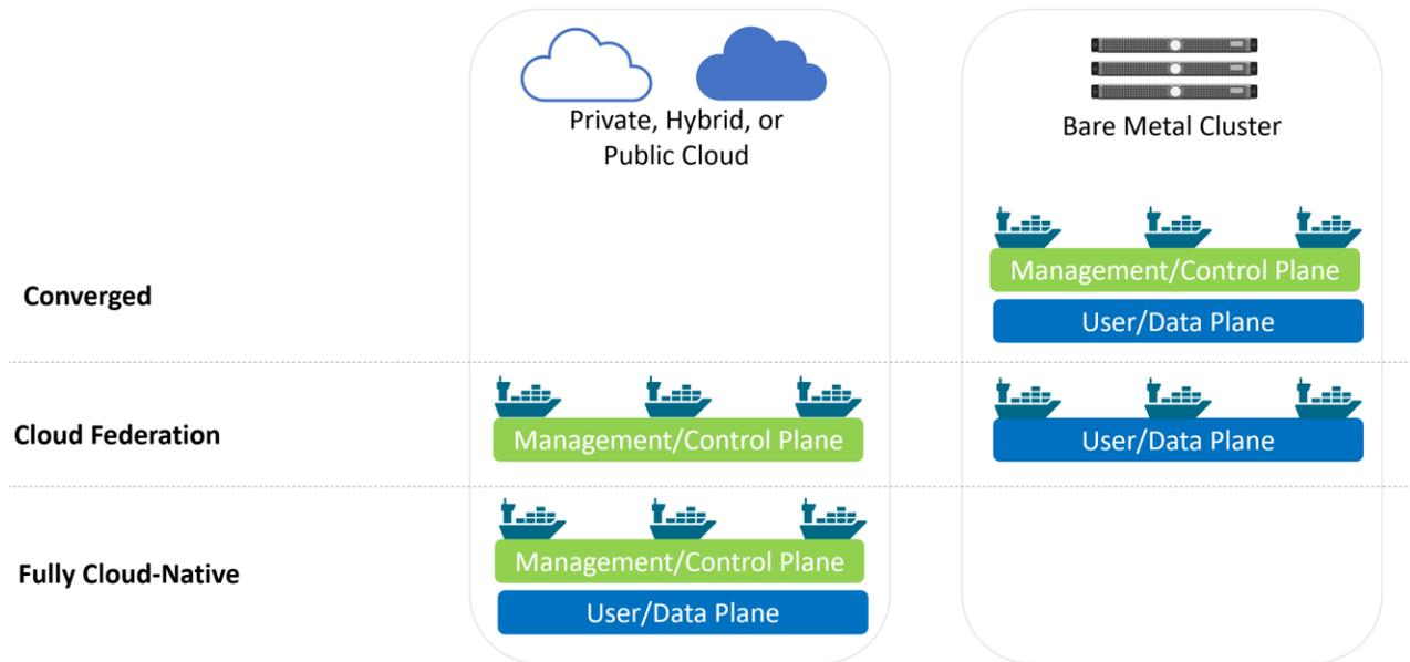
Figure 2 – Entra vCMTS Deployment Models
