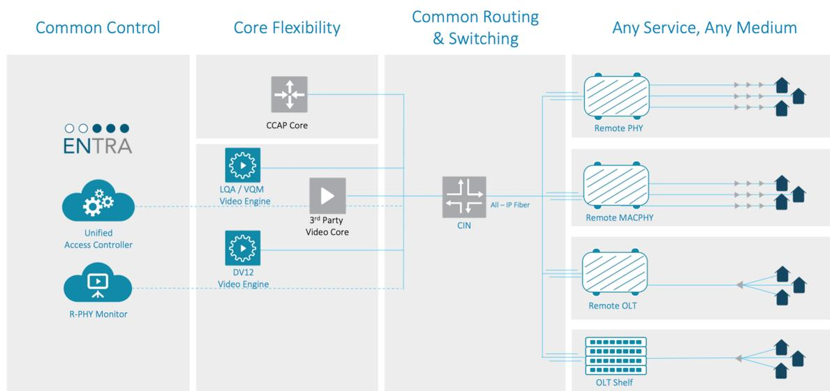
SF-4X Access Node is a sealed remote optical line terminal (R-OLT) with four 10 Gb/s Ethernet Passive Optical Network (EPON) ports and up to four 10 Gb/s Ethernet uplinks. With support for DOCSIS® Provisioning over EPON (DPoE™), the SF-4X Access Node provides cable operators with a fiber to the home (FTTH) solution and is an essential component of the Entra unified cable access solution.
